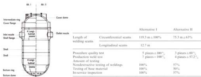
Fig. 13 Reduction number of welds and tests when increasing the size of forgings. [30]
