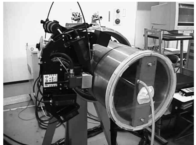
Fig.15 An example of small automatic welding system.[11].
